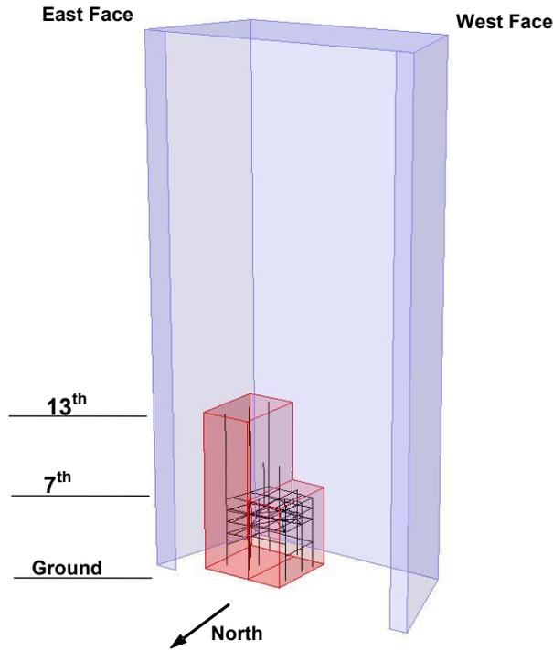
Figure L-30. Likely region of initiating component failures based on videographic and photographic records of fire and collapse.
