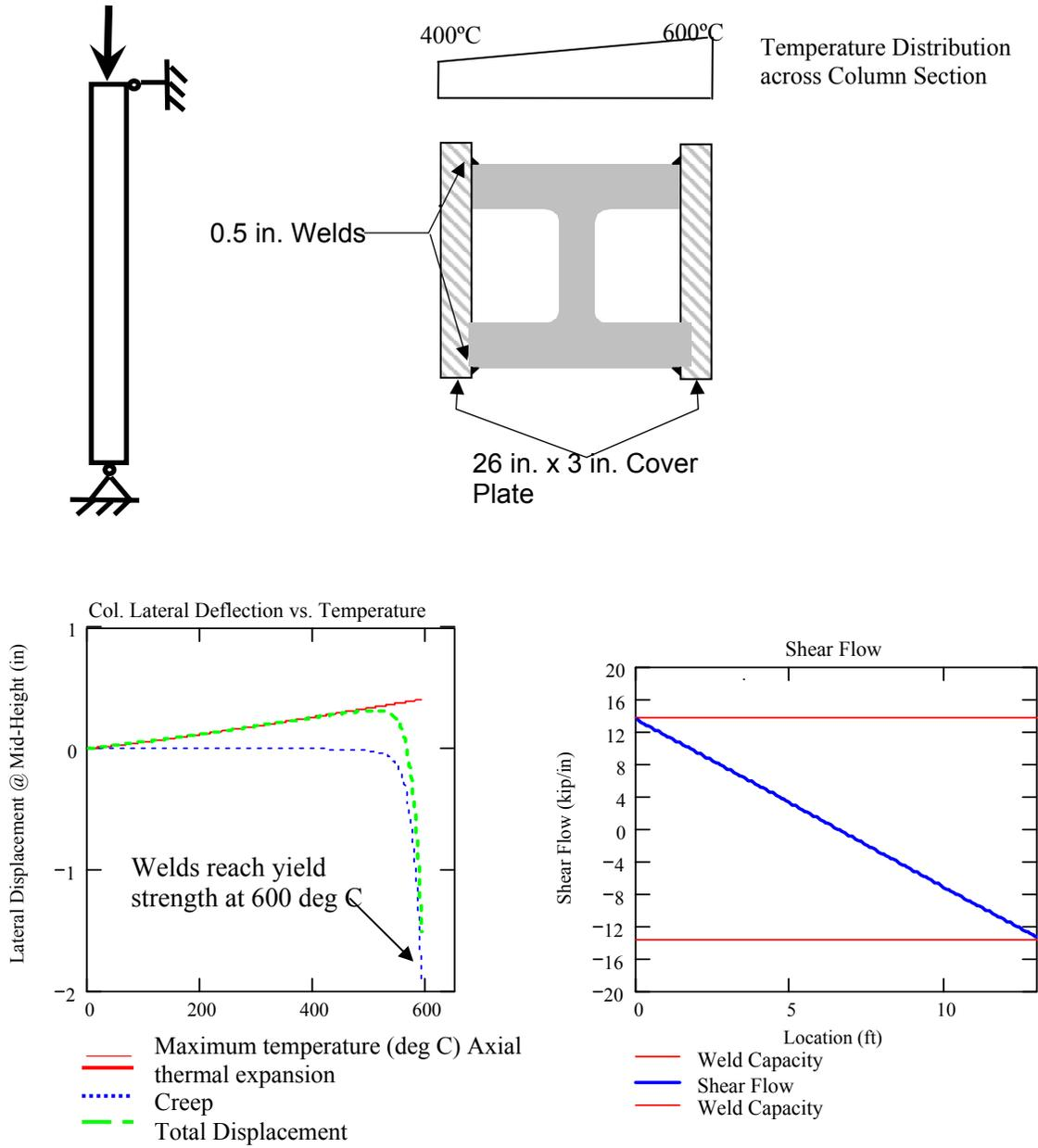
**Figure L-38. Effects of temperature gradient on interior column 79.**
