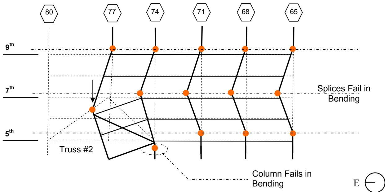
**Figure L-49. Horizontal progression mechanism for truss #2 failure.**
