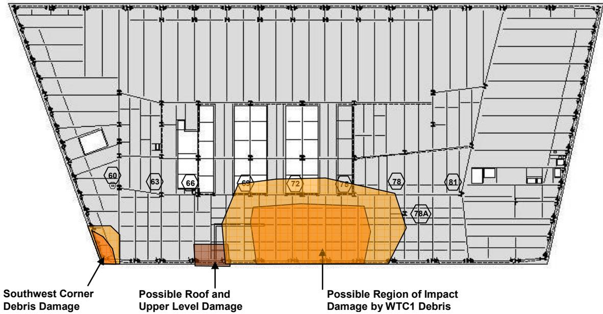
Figure L-23c. Possible extent of debris damage in plan.
