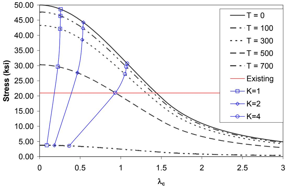
Figure L-37. Column 79 capacity versus temperature and unbraced length K.
