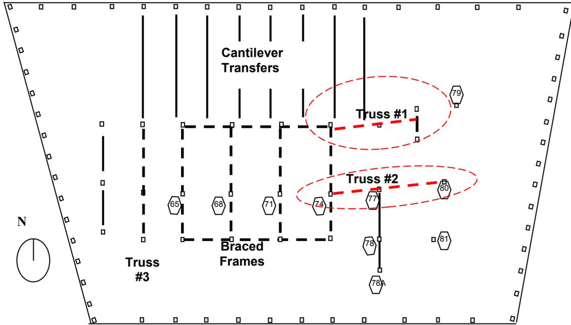
Figure L-47. Transfer components between Floors 5 and 7.
