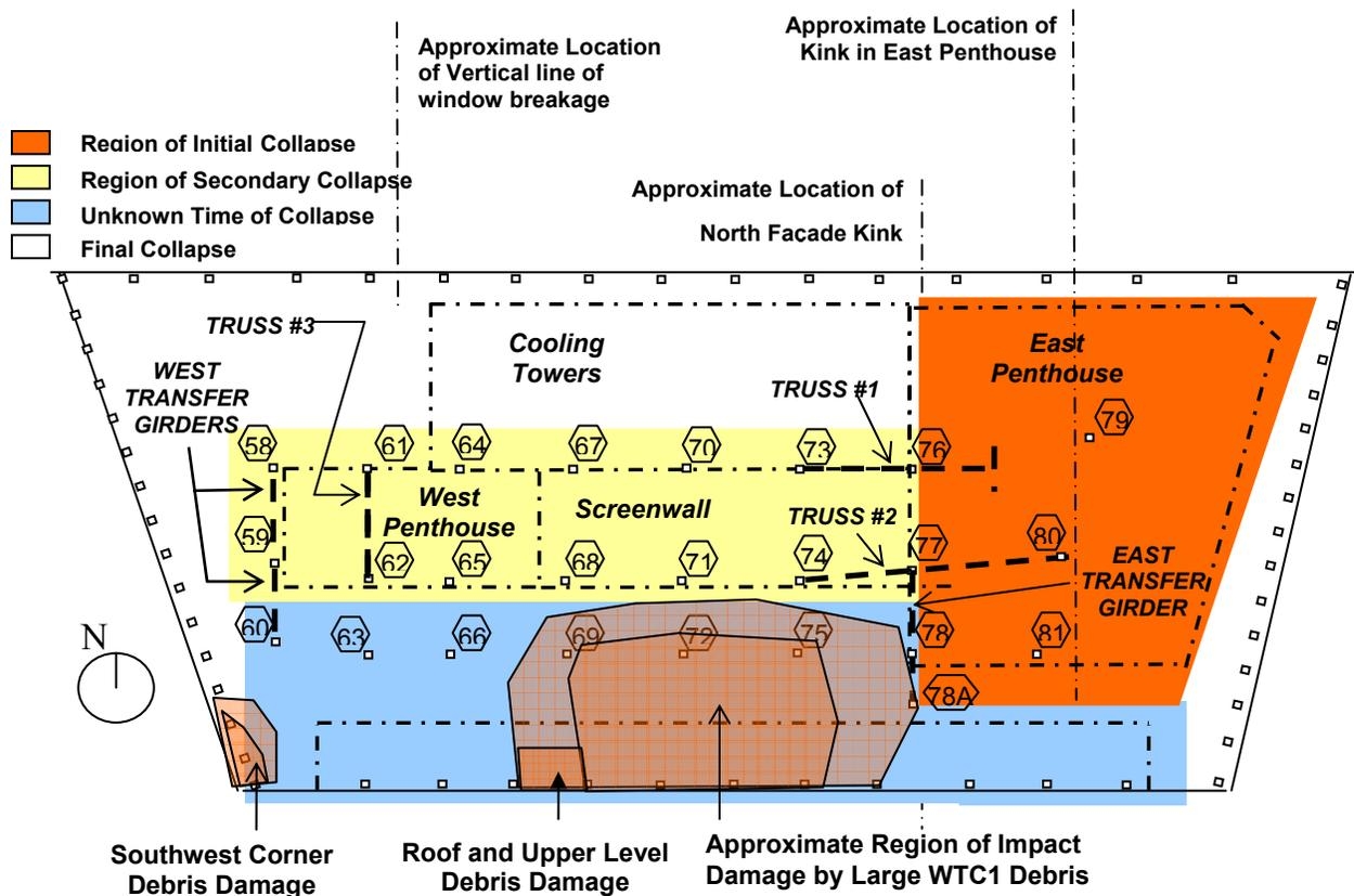
Figure L-31. Plan View of Collapse Progression.
