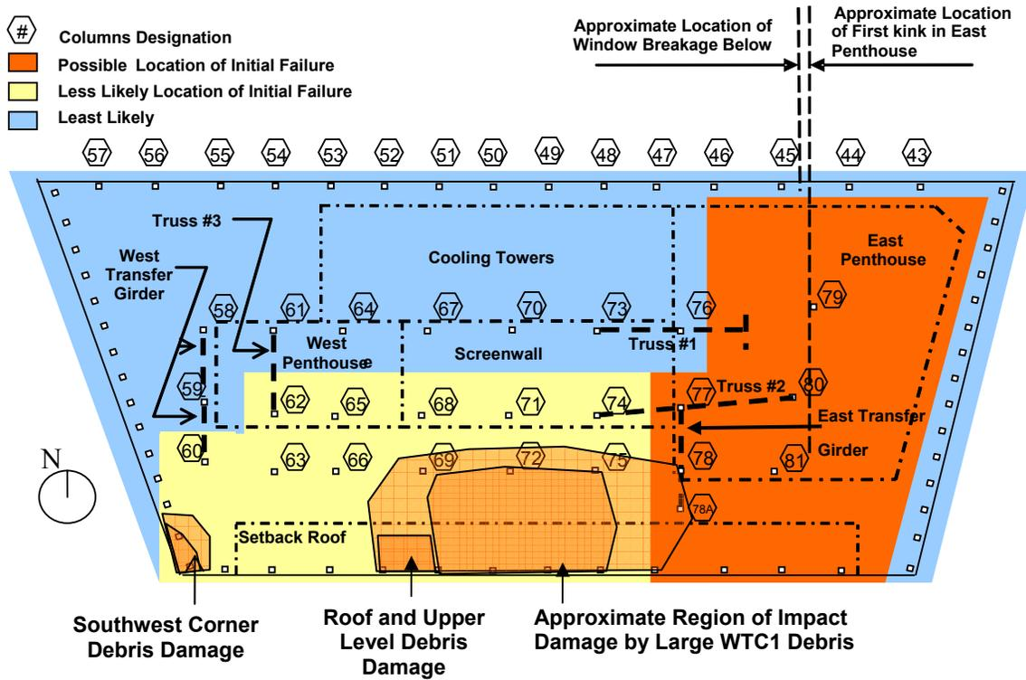
Figure L-29. Plan view of regions for collapse initiation.
