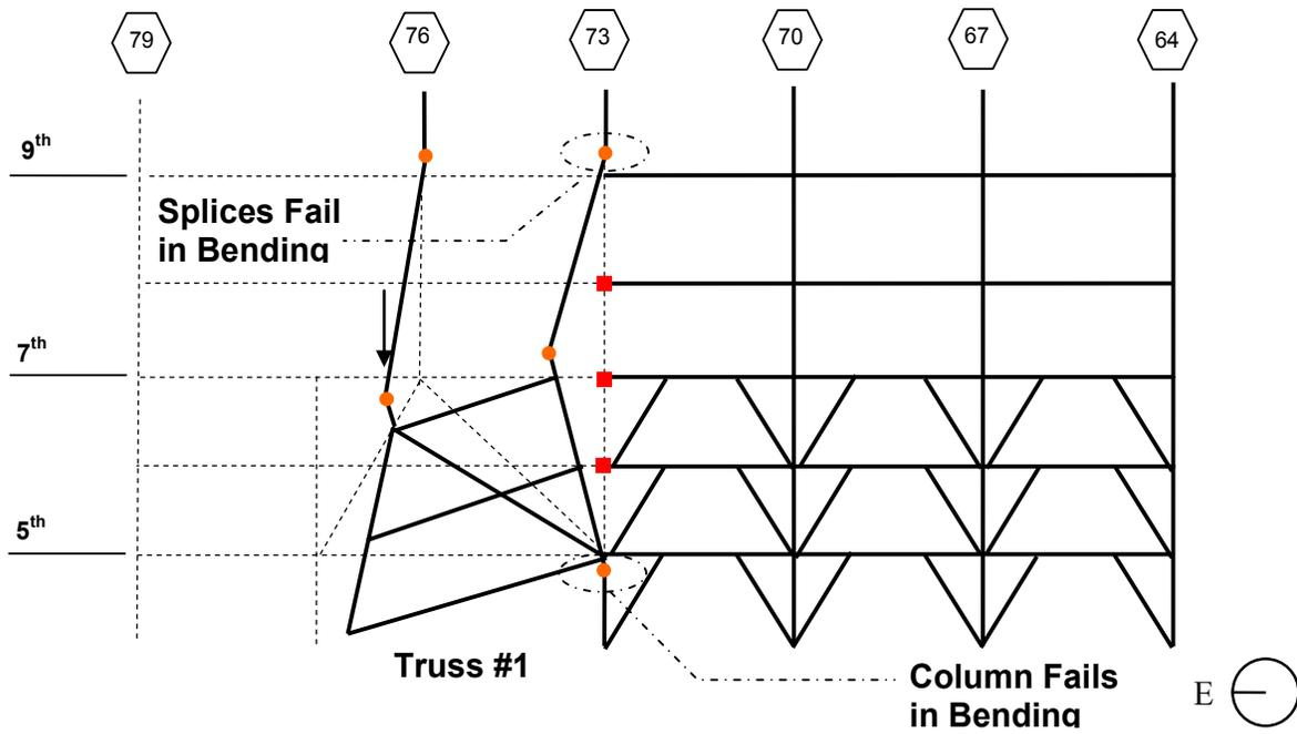
Figure L-48. Horizontal progression mechanism for truss #1 failure.
