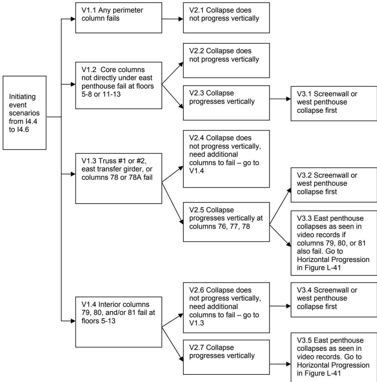
**Figure L–40. Vertical collapse progression scenarios.**
