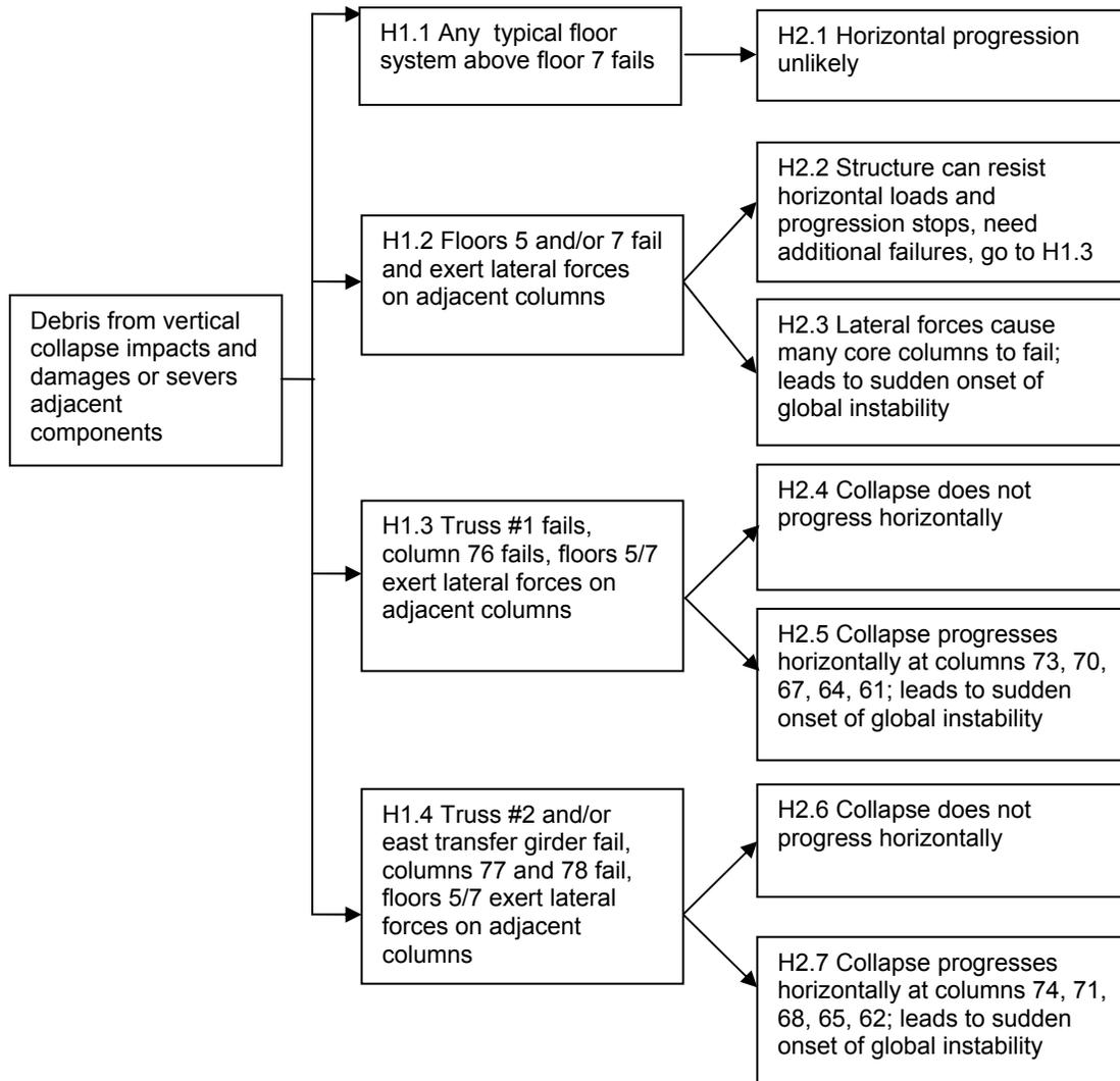
**Figure L-46. Horizontal collapse progression scenarios.**
