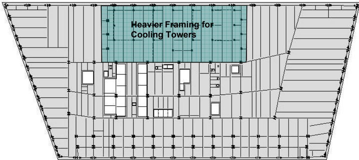
Figure L-14. Floor 46 plan.
