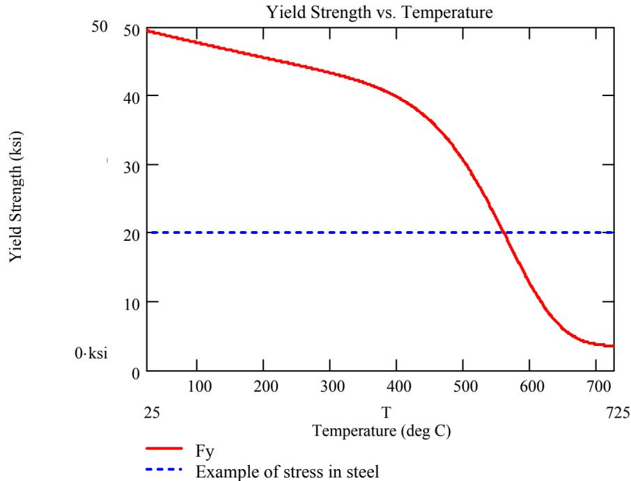
**Figure L-39. Steel strength versus temperature.**
