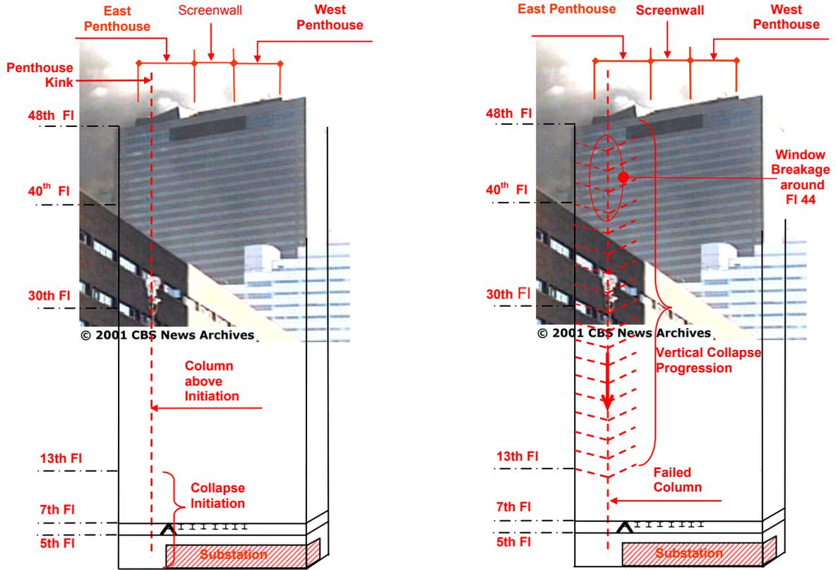
Figure L-33. Collapse initiation and vertical progression on the east side of WTC 7.
